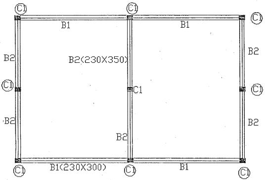
Grid of Column is 6MX6Mc/c in Both Direction SLAB-125 MM THK.
