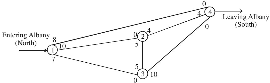
What is the maximal flow of vehicles per hour through the system ?
